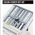
Color-coded fold plate graphics ensure accurate placement of paper stops.
