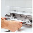
The blade changing device covers edge of blade for safe handling.
