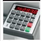
The "EP" back gauge control module features a digital display and keypad for programming.
