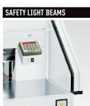
Safety light beams protect the operator and allow back gauge to automatically advance to the next cut.
