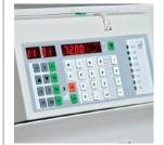
The back gauge control module has a digital display and keypad for programming.
